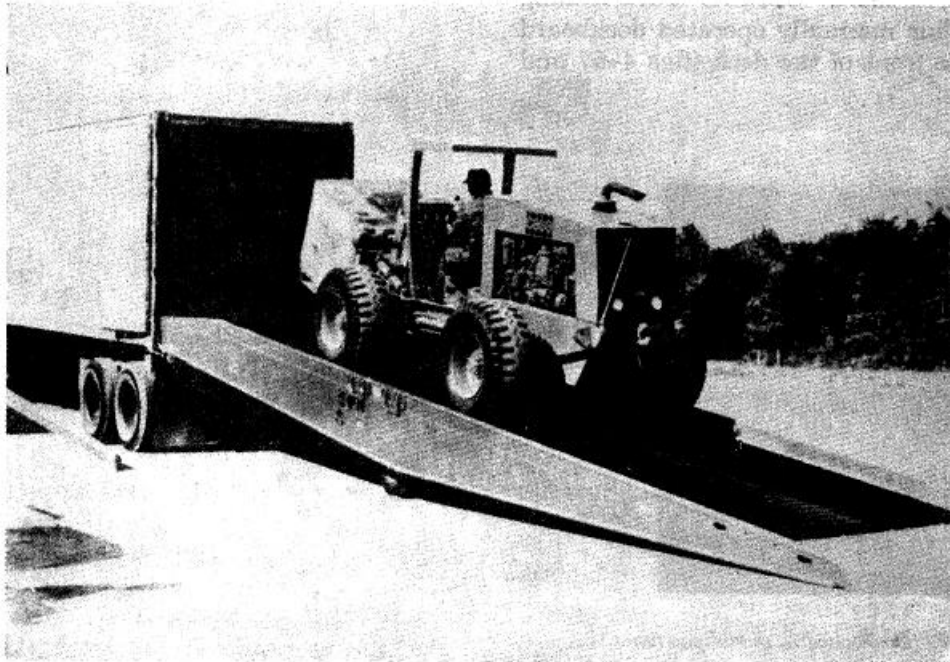
Figure 4-69. Mobile vehicle loading ramp.
