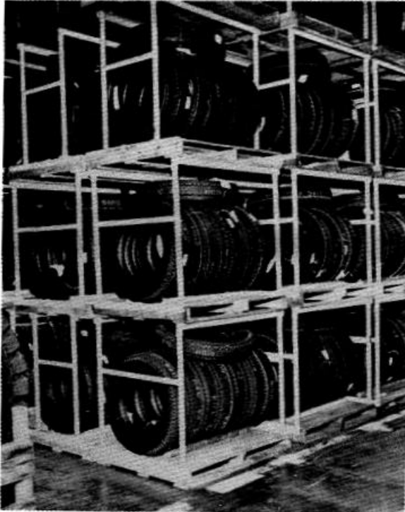
Figure 4-96. Support sets used for tire storage.
