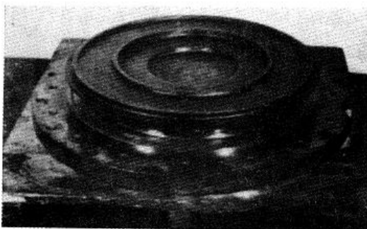
Figure 5-74. Cable dispensing turntable.
