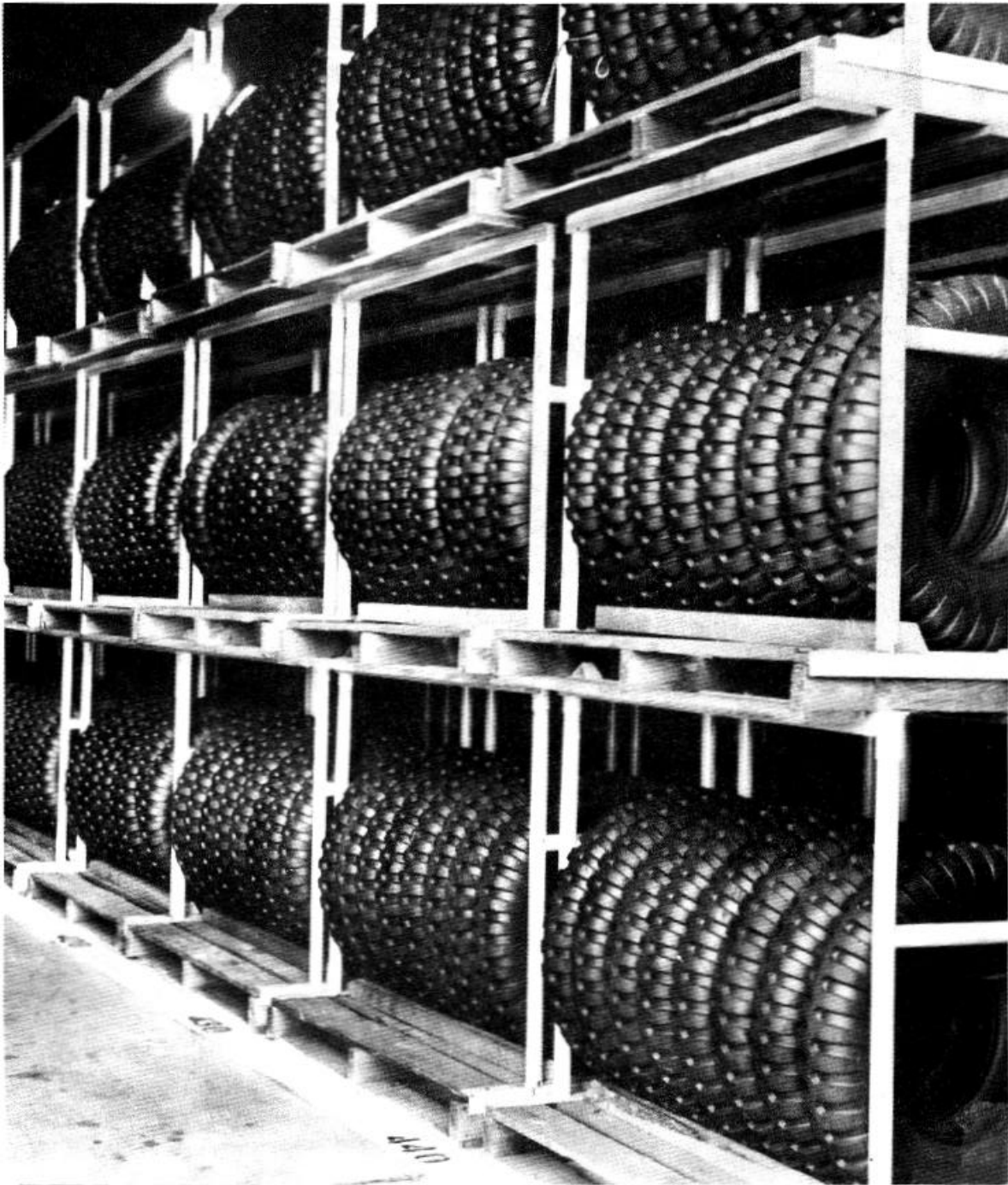
Figure 5-43. Typical storage in pallet support sets.
