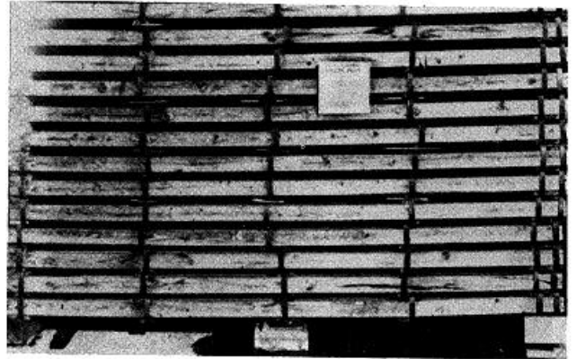
Figure 5-65. Strapped bundles of steel in open storage.
