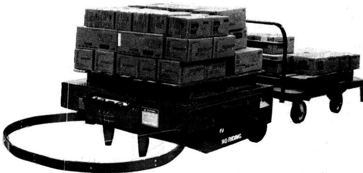
Figure 4-31. Trailer, platform, warehouse, 4,000- or 6,000-pound, towed by driverless tractor system:
